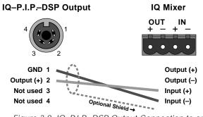
Figure 3.8 IQ–P.I.P.–DSP Output Connection to an IQ Component with a Screw Terminal Plug Connector
